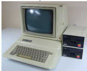
Operating system Apple DOS 3.3, ProDOS CPU 6502 @ 1.023MHz Memory 64 KB RAM (up to 1 MB)
